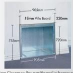
Zero Clearance Box positioned in framework mounted on 18mm Villa Board cut out size. (Box size: 905w x 720h) (Cut out size: 905w x 755h)
